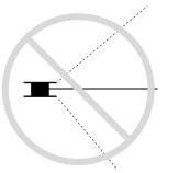
Properly mounted reel pivots or swings as cord or hose travels side-to-side. Straight pull off reel improves operation, increases life of reel and cord or hose.
