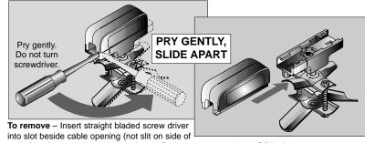
trolley) and pry gently as shown above. Do not turn screwdriver. Slide Apart
