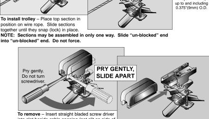
into slot beside cable opening (not slit on side of trolley) and pry gently as shown above. Do not turn screwdriver. Slide Apart
